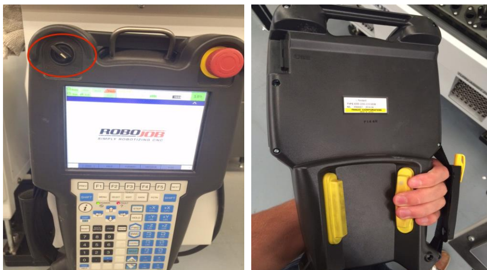
Picture 51 - Switch and dead man's button on de Teach Pendant
