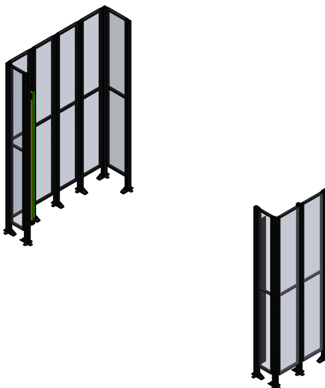
Figure 2.10. Safety fence with safety light curtain
