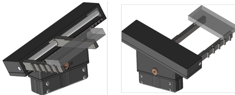
Figure 3.32. Revolving unit with shifted origin
