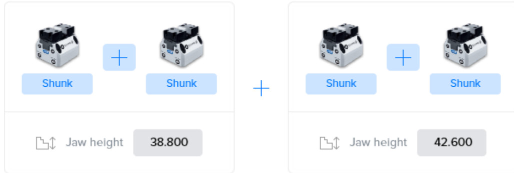
Figure 3.26. Configuration with two sets of two combined fixtures
