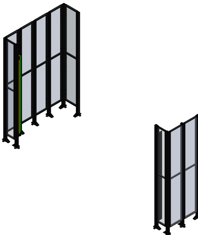
Figure 2.25. Safety fence with safety light curtain
