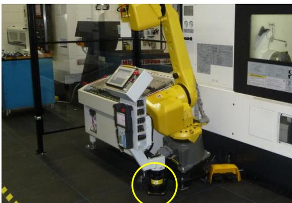
Figure 17.3: Positioning Laser scanner
