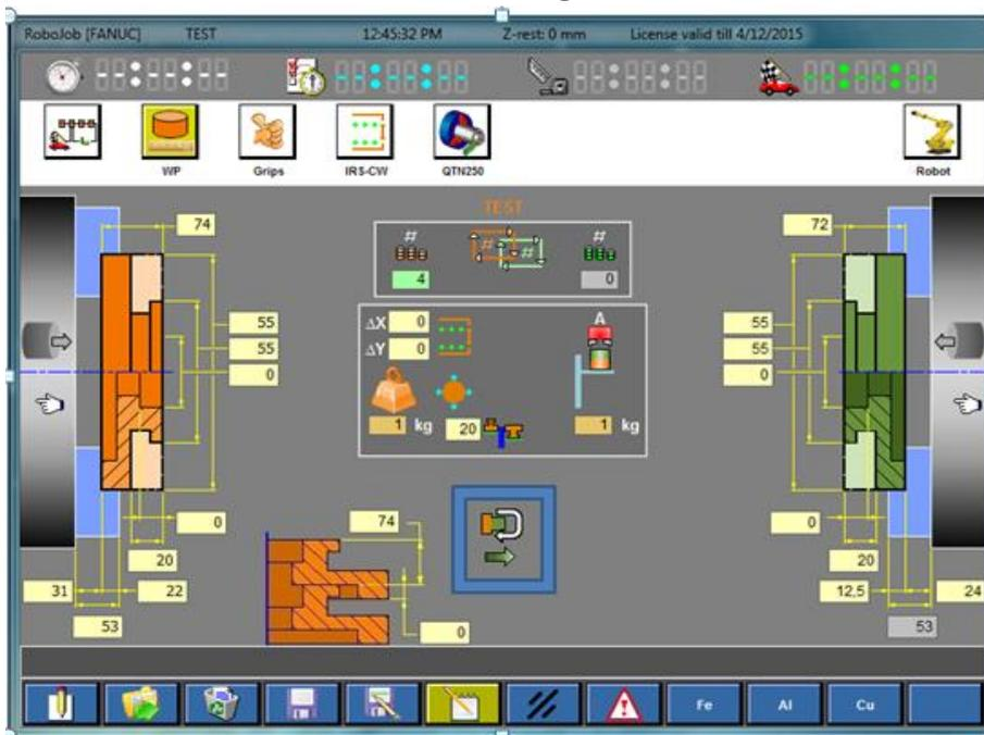
Figure 13.5: Rotational unit icon (activated here) in the WP sub-screen
