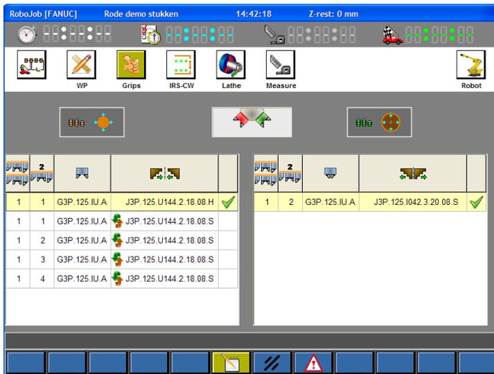
Figure 4.2: Gripper sub-screen with Gripper magazine
