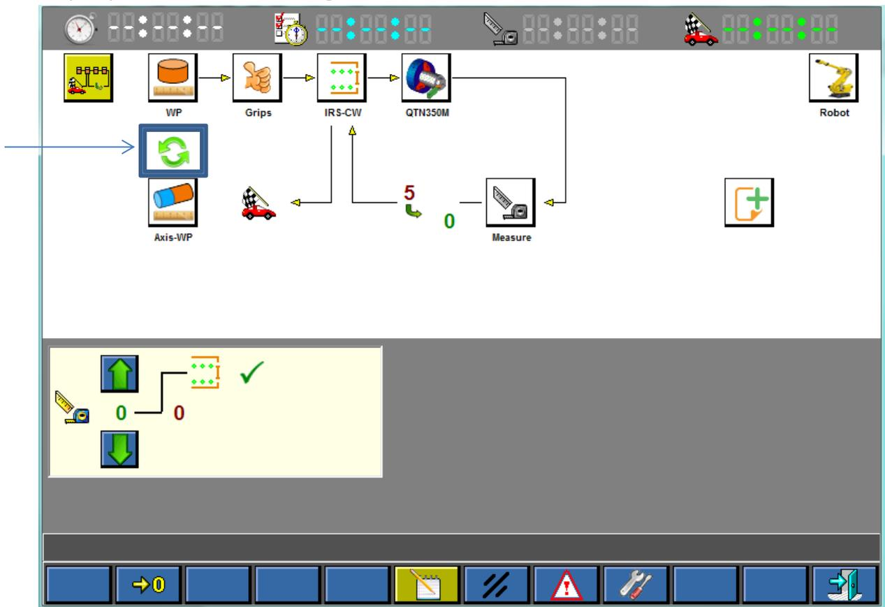
Figure 14.1: Software for switching shafts/discs
