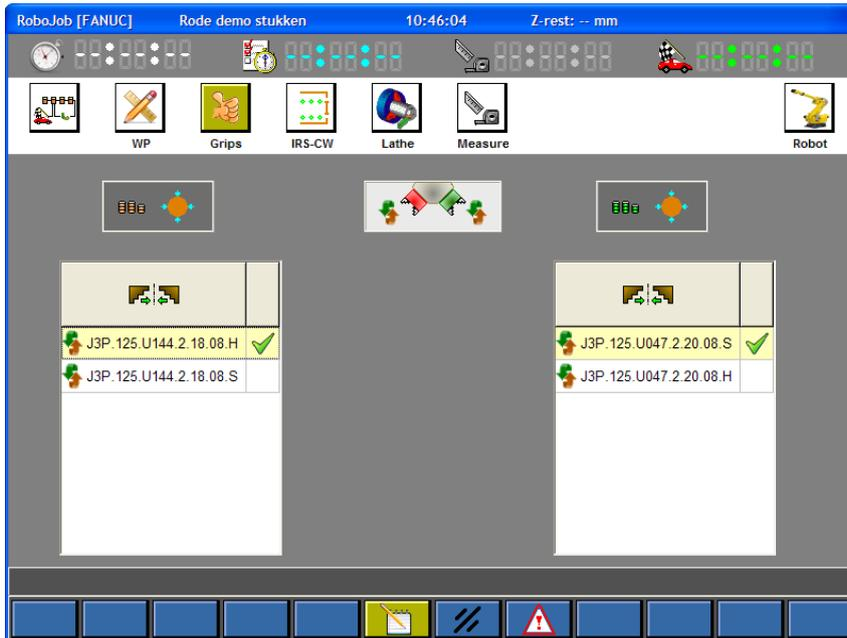
Figure 4.6: Gripper sub-screen without Gripper magazine
