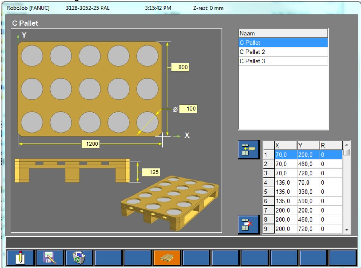
**Figure 12.7: Calibre pallet settings screen**
