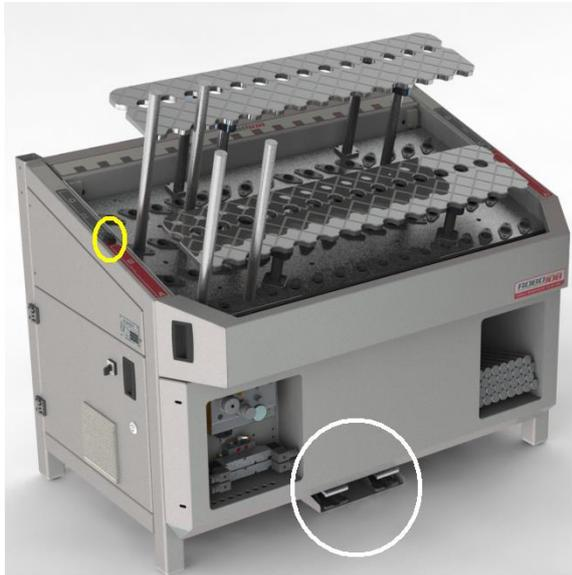
In order to select which IRS-CW plate has to be operated by the foot pedals, we make use of the selector switch, indicated in the yellow circle in fig. 5.7.
