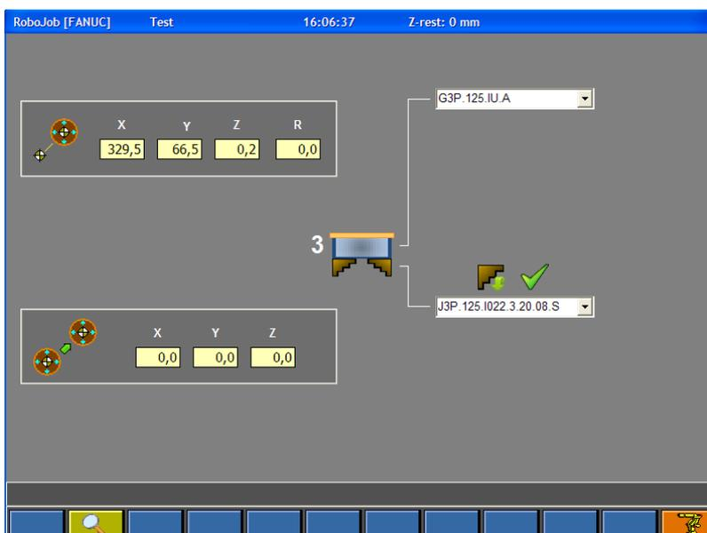
Figure 2.18: Adding gripper to the gripper magazine
