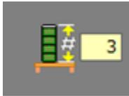
The stacking height of the pallet may be specified as desired, but with a safety maximum that is determined on installation of the system. The desired height is expressed in the number of stacked workpieces.
