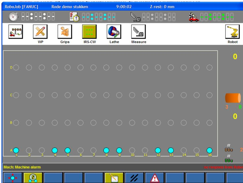
As shown in fig.15.1 we can differentiate between the alarms that are displayed to the left and the alarms that are displayed to the right. The alarms on the right are alarms that relate to the communications. These alarms are not shown in the alarm list.
