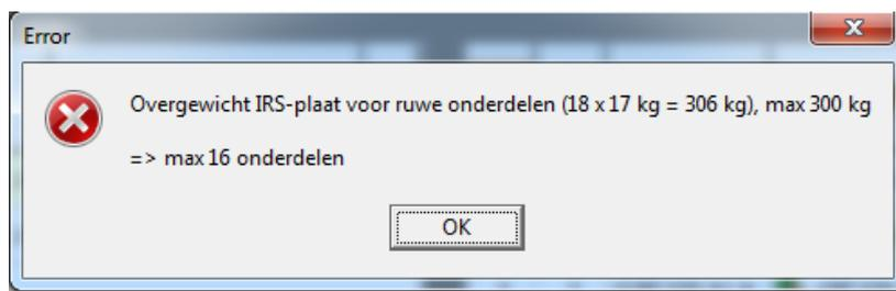
Figure 3.8: IRS plate overweight error message
