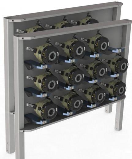
Figure 2.8: Gripper magazine
