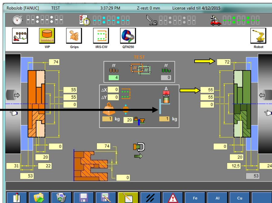
Figure 13.10: First rotational unit setting screen
