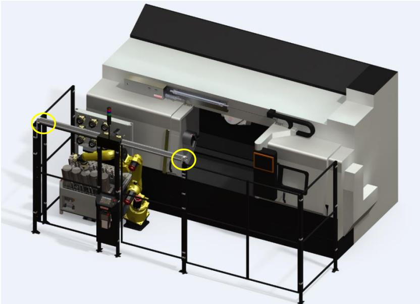
Figure 17.5: Installation with safety fencing and 2 doors
