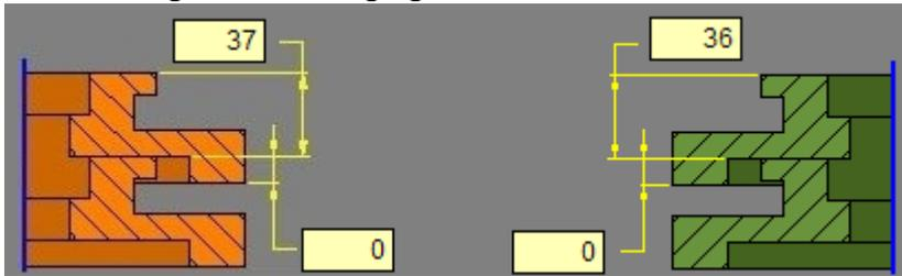
Figure 3.10: Interlocking workpieces
