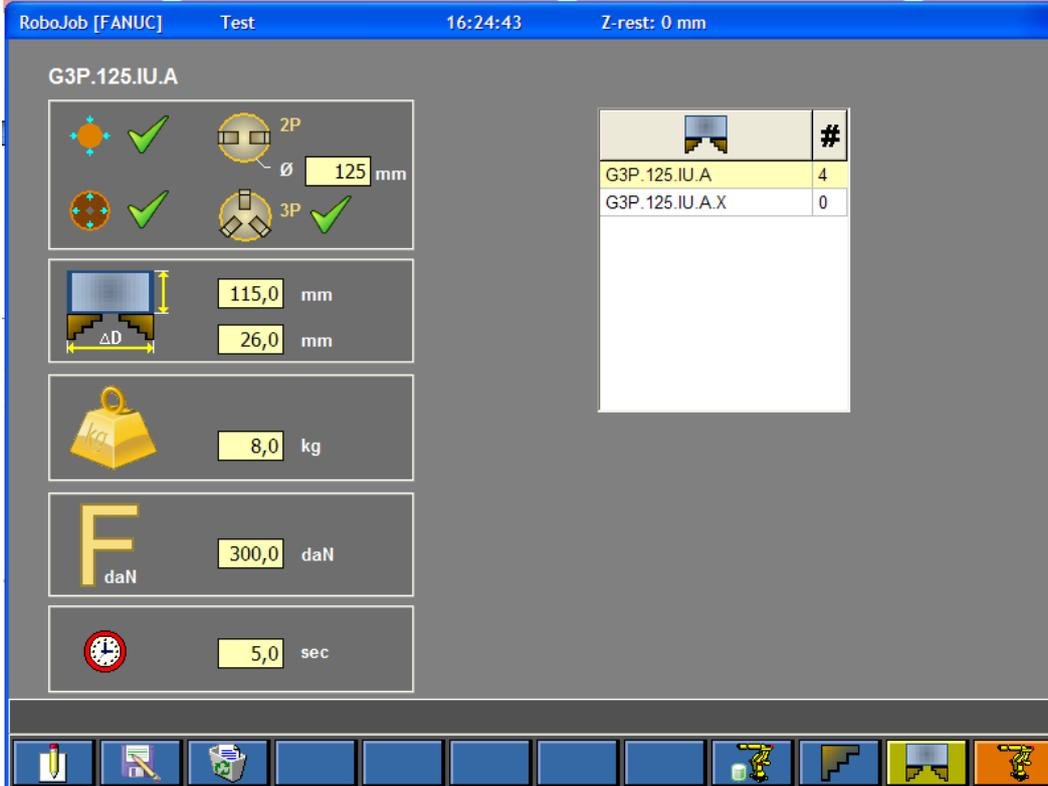
Figure 2.19: Sub-gripper properties 1
